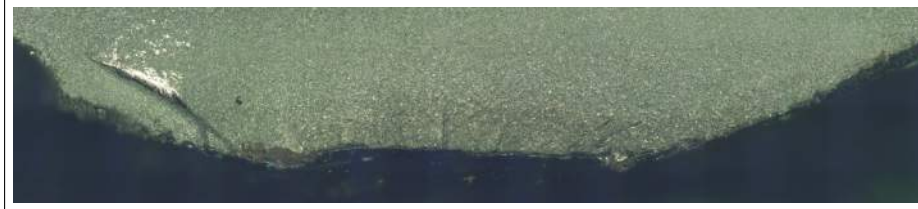
(c) Picture of crack initiation site for specimen 10 from optical microscope.
