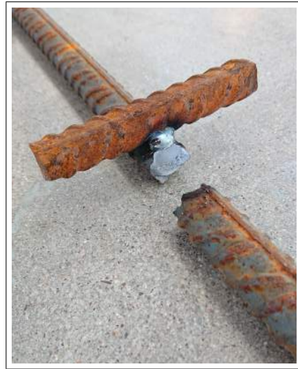
(b) View of separation of specimen 1.
