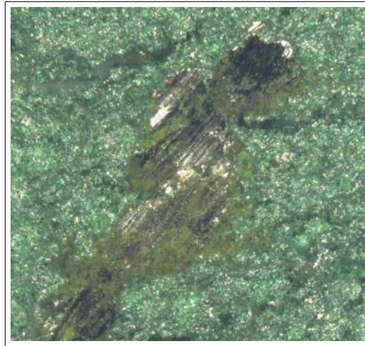
(d) Captured banded structure from center of fracture surface of specimen 10.
