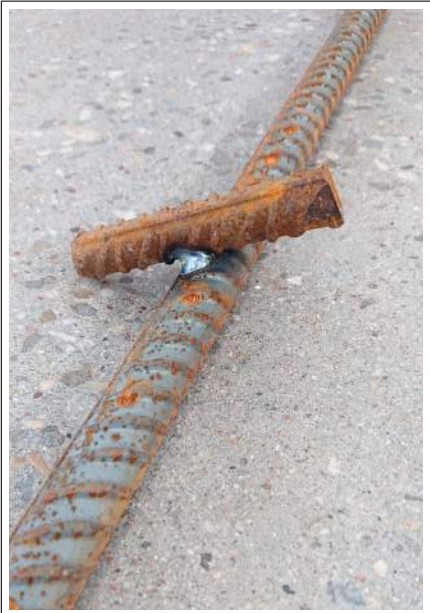
(b) Picture showing spot weld.
