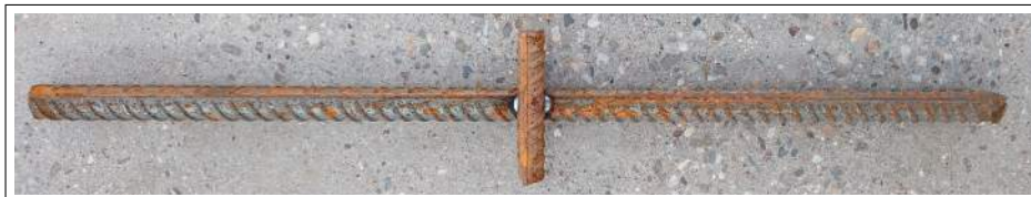
Figure 1.2: Overview of a specimen showing the as received status with limited corrosion.
